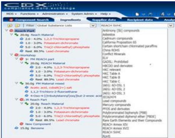
With the aid of the **filter function**, here e.g. **REACH SVHC**, you can find out quickly and simply whether your product contain substances from the filtered list, as these are marked with a color on the bill of materials (BOM).
