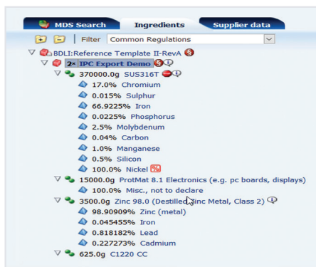
Figure 2. Parallel reality: Assemble supplier products to build your product. Enhance your product in CDX with value-added content to make it ready to report via export with specific scope in formats such as IPC-1752A, IPC-1754 or IEC-62474, or integrate CDX with in-house systems.
